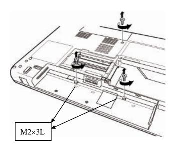
Figure 4-11 Removing the screws securing keyboard
